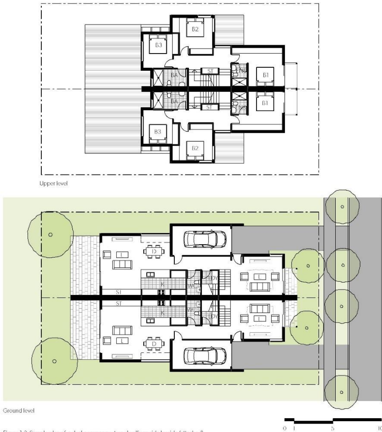
Figure 1-8. Sample plan of a dual occupancy - two dwellings side by side (attached)
